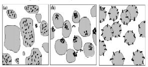
**Fig: 6.** Schematic depictions of CNTs and Al powder after different mixing techniques. In (a) high energy ball milling, CNTs were effectively dispersed though insufficiently distributed within the Al powders; and in (b) low energy ball milling, CNTs dispersed within Al powder though agglomerates still existed; and in (c) the PBA method, CNTs were coated with Al powders though agglomerates still existed. [10]
