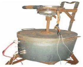
Fig: 5. Stir Casting Unit [7]
